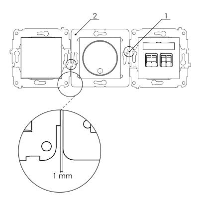
1. First, install the electronic light control mechanism in the mounting box. The other adjacent mechanisms are installed so that the "dovetails"(1) (if any) overlap the central plate of the controller (2).
